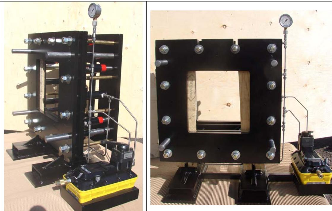
Hydraulic target retention clamping test frames are superior to conventional test frames for air back V50 fragment testing. The hydraulic clamping frames provide consistent, even tension and pressure through the test article. This type of frame is better suited for fragment testing than bullet testing. Uses standard shop air supply (90 psi) for activation.
